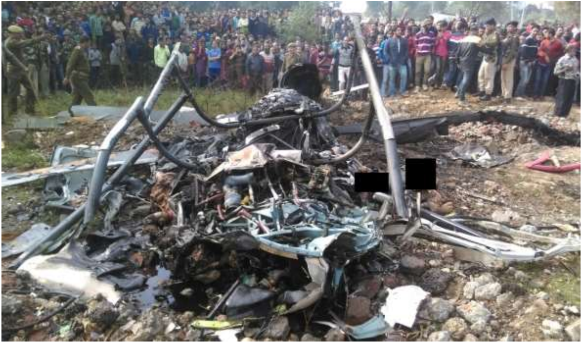
Helicopter lying upside down with skids facing upwards (Final resting position)
