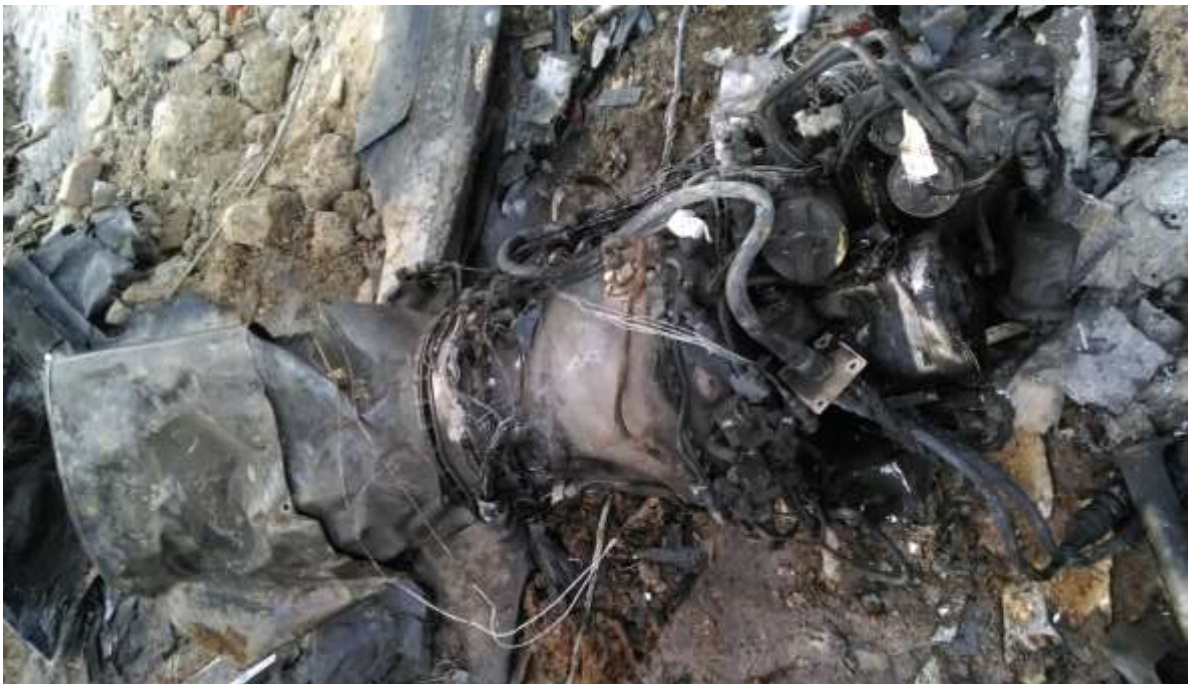
Damaged and externally burnt engine
