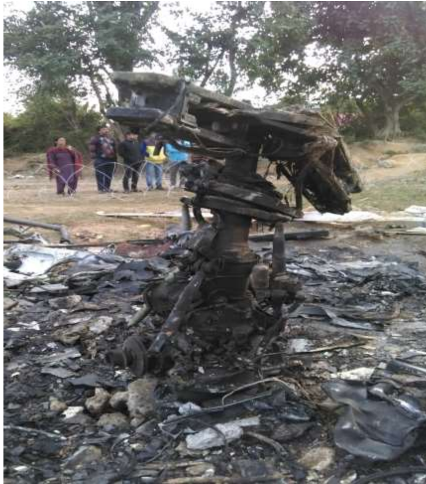
Damaged Main Rotor Gear Box
