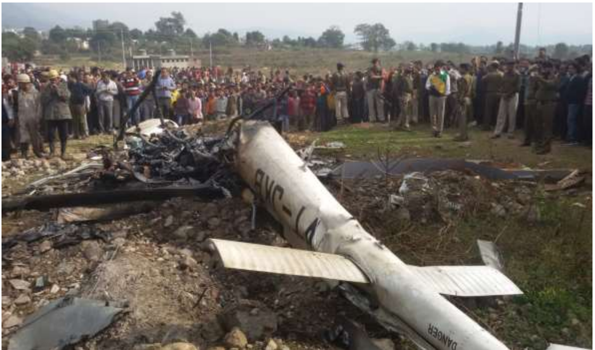
Damaged Tail boom (severed from the burnt fuselage).
